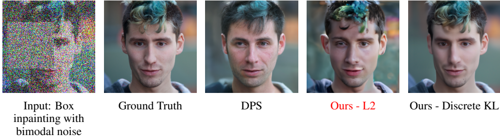
Figure 3: Results on the box inpainting task with a bimodal noise distribution. By optimizing the discrete KL divergence, we can reconstruct the face with much higher fidelity than existing methods like DPS or our method with L2 loss.
