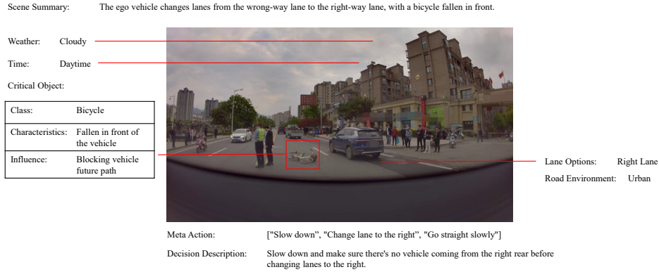
Figure 8: An example of overturned bicycles and motorcycles in the SUP-AD dataset. A bicycle has fallen in front of the ego vehicle, requiring the ego vehicle to change lanes.
