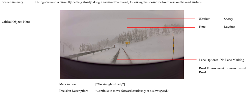
Figure 13: An example of snowfall in the SUP-AD dataset. Most of the road is covered by snow, requiring the ego vehicle to move forward cautiously by following the snow-free tire tracks.
