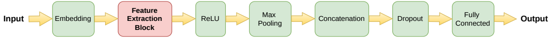
Figure 1. Common model architecture used across all experiments. The Feature extraction block represents different feature transformation strategies across six model variants.
