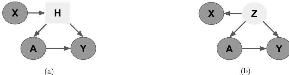
Figure 5: Causal Graph - (a) Deterministic Representation: H corresponds to a hidden layer representation that is a deterministic variable, X is a covariate, A is an action, and Y is an outcome variable. (b) Stochastic Representation: Z is a latent variable, X is a noise version of confounder Z , A is an action, and Y is an outcome variable.
