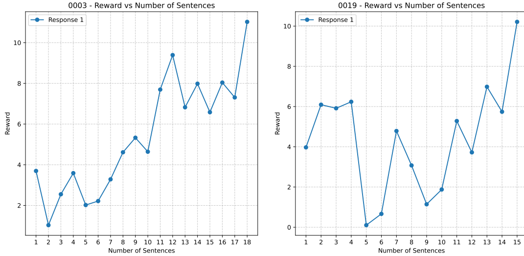
Figure 5: Reward vs # Sentence plot for Llama3-8B Model. It shows the reward change as the response is generated.
