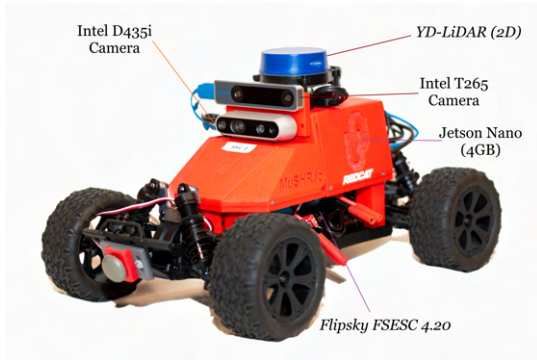
Fig. 5: ARC with detailed view of onboard sensors and processor.
