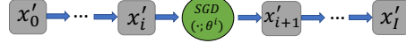
Figure 2: Iterative solvers for data reconstruction attacks as unrolled deep feed-forward networks: We map the i -th SGD iteration (parametrized by \theta^i ) into a single network layer, and stack I layers to form an I -layer deep network. Feeding forward data through the I -layer network is equivalent to executing I SGD updates. The trainable parameters \{\theta^i\} are colored in blue. These parameters can be learned from real (reconstructed) data by training the deep network in an end-to-end fashion.
