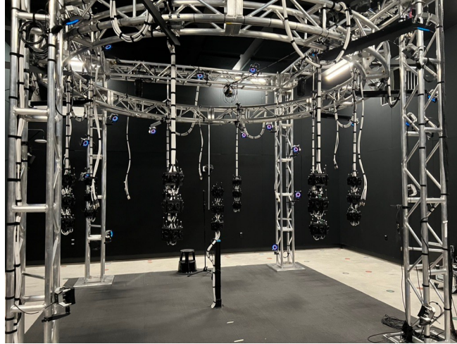
Figure 9. The large-scale binaural data capture system with artificial binaural heads.
