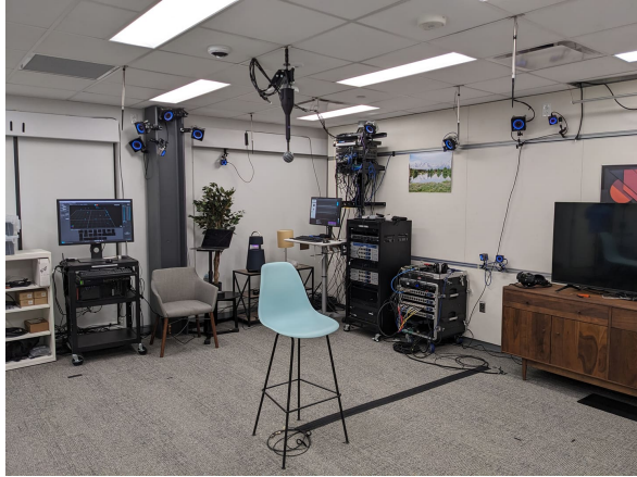
(a) We collect data in a standard room without significant soundproofing or sound-absorbing materials. The background noise from multiple air conditioning vents and electronic equipment is recorded.
