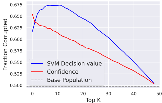
Figure 19: The fraction of ImageNet-C test images that are corrupted with Gaussian noise when ordering the images by either their SVM decision value or by the model’s confidences, averaged over all classes. Our framework more reliably captures the corruption than using confidences.
