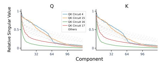
Figure 10: Sorted relative singular values of  $W_Q$  and  $W_K$  for each QK circuit at pythia-160m layer 5. Each circuit shows strong alignment between the spectra of  $W_Q$  and  $W_K$ , suggesting similar structural properties. Circuits 4 and 15 have relatively high effective rank, while Circuits 16 and 17 exhibit significantly lower rank.
