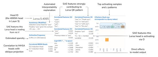
Figure 4: Visualization dashboard for a "you"-specific induction Lorsa head. We provide an example interpretation of each item below.
