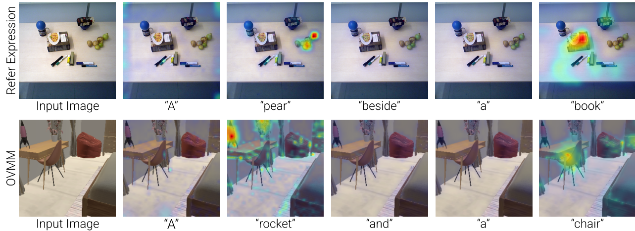
Fig. 8: The Stable Diffusion model allows us to extract word-level cross-attention maps for any given text prompt. We visualize these maps in a robotic manipulation environment and observe that they are accurate at localizing objects in a scene. Since these maps are category agnostic, downstream policies should become robust to unseen objects at test time.
