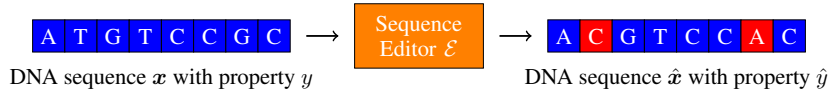
Figure 1: An example of editing the DNA sequence ‘ATGTCCGC’. The goal is to make a limited number of edits to maximize the property \hat{y} . Each token in the sequence in this example is called a base and can be any one letter from the alphabet [‘A’, ‘C’, ‘T’, ‘G’]. The editor function \mathcal{E} accepts the starting sequence and determines that the second and seventh bases require editing (highlighted in red). Then, \mathcal{E} modifies the bases at these identified locations.
