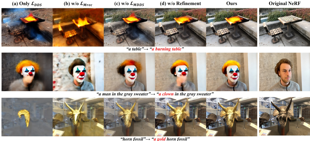
Figure 5: Ablation studies. (a) If we only use DDS loss, the model fails to maintain the attribute of untargeted regions and often fails to reflect text conditions. (b) If we do not use masked reconstruction regularization, again the regions beyond the target objects are excessively changed. (c) If we remove the mask from DDS, unwanted artifacts occur in untargeted regions. (d) With removing the proposed refinement layer, the results become blurry as the backbone NeRF cannot fully embed real-world scenes. Our proposed setting can modify a specific region in a 3D scene and follow the target word without causing unwanted deformations.
