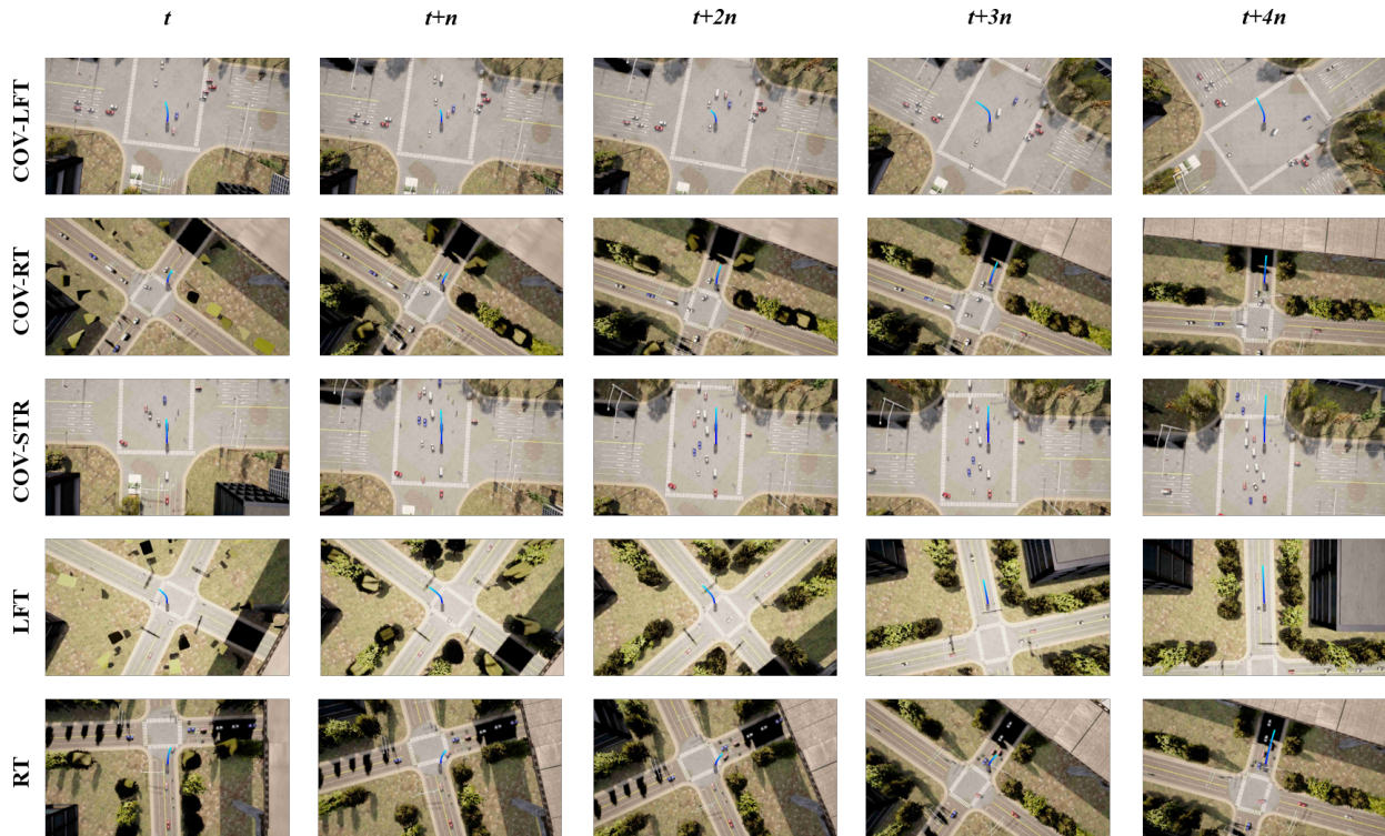
Figure 8: Five Sub-scenario Driving Behavior Visualization: This visualization encompasses five driving scenarios: competing with other vehicles while turning left (COV-LFT), turning right (COV-RT), and going straight (COV-STR), as well as normal left turns (LFT) and right turns (RT). Frames are sampled at intervals t , t+n , t+2n , t+3n , and t+4n from the driving sequences to depict the vehicle’s behavior over time. Each image is presented from a top-down view , with the ego vehicle (depicted in gray) centrally positioned. The vehicle’s motion direction is represented by a purple trajectory line.
