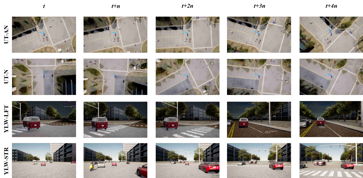
Figure 10: Four Sub-scenario Driving Behavior Visualization: This visualization encompasses four driving scenarios: U-turns in abnormal (UT-AN) and normal conditions (UT-N), and passing through yellow lights while turning left (YLW-LFT) or going straight (YLW-STR). Each image is presented from a top-down view or front-head view.
