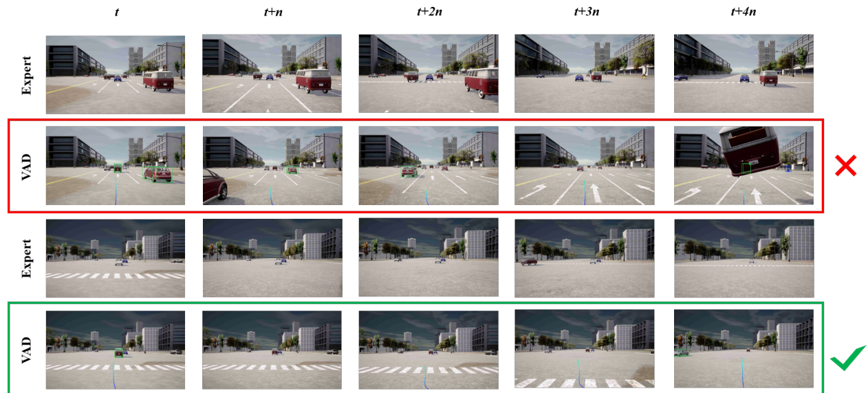
Figure 16: Successful and Failed Cases in the STR Scenarios: In the failed case, the ego vehicle controlled by the trained VAD model accelerated slowly while traveling straight and collided with a replayed trailing vehicle. Under the same replay protocol, the successful case traversed the intersection without collision.
