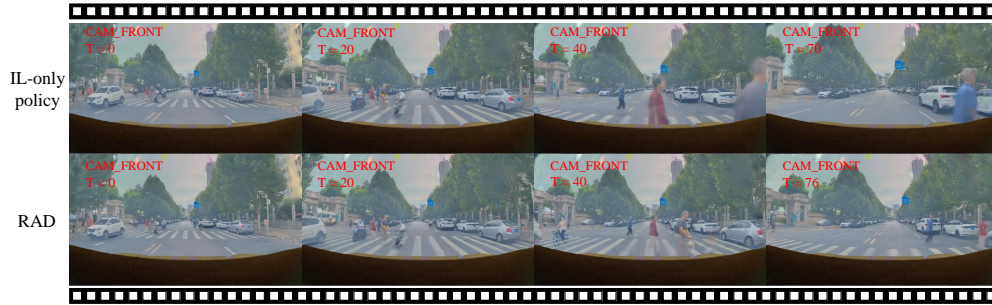
Figure 6: Closed-loop qualitative comparisons between the IL-only policy and RAD in a Yield to Pedestrians scenario. The IL-only policy fails to yield (Row 1), while RAD successfully yields to pedestrians (Row 2).
