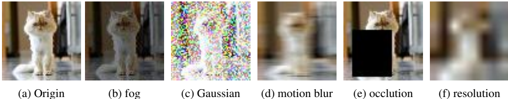
Figure 8: Illustration of the image corruption types, including fog, Gaussian noise, motion blur, random occlusion, and resolution.
