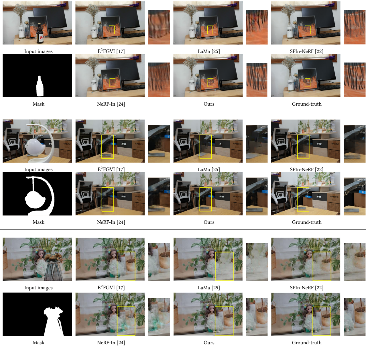
Figure 6: In the 3D inpainting task, we provide a qualitative comparison between our method and baseline methods in our proposed dataset.
