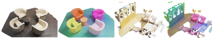
Figure 14: Learned backbone features. AGILE3D learns general object-level features. The point features are projected to RGB space using principal component analysis (PCA).
