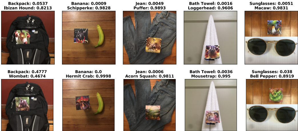
Figure 6: Successful examples of universal, physically-realizable feature-fool attacks (top) and pixel-space attacks (bottom). See Appendix A.6 for full-sized versions of the patches.
