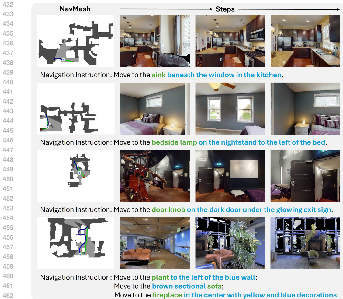
Figure 5: Examples of visualized trajectories and observed images. In the navigation mesh (NavMesh), the color green denotes the reference path, while blue indicates the actual path taken by the agent.
