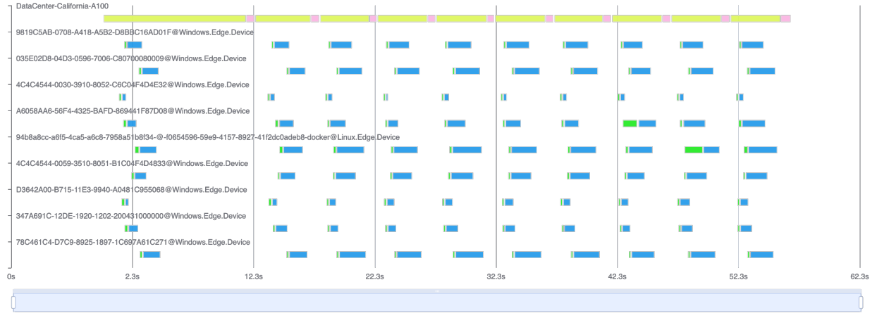
Figure 12: Real-world application demonstration. Yellow: aggregation server waiting time; pink: aggregation time; green: client training time; blue: client communication time.
