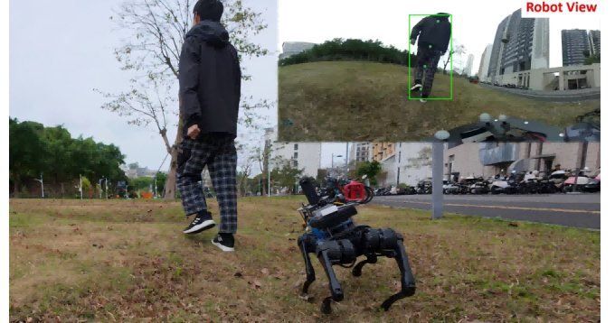
Fig. 1. A scenario of a quadruped robot following a person through a rugged lawn. The robot view is from an onboard panoramic camera (see Sec. IV-C). The robot’s dynamic motion induces severe camera ego-motion and vibration, which bring challenges for person localization.
