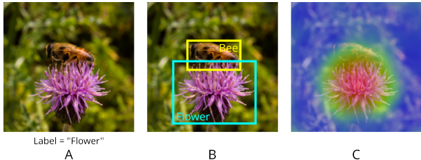
Figure 5: Illustration of Image Classification (A), Object Detection (B) and Class Activation Mapping (C). In (A), a (hypothetical) model has assigned the label “Flower” to the image. In B, a (hypothetical) Object Detection model has detected one instance of “Flower” and “Bee”. In C, a (hypothetical) CAM output is superimposed on A, showing what parts of the image contributed to the model assigning the label “Flower”. The redder the pixel, the more it contributed.
