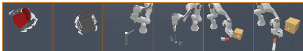
Figure 4. Sampled geometric variations for Push Chair, Turn Faucet, and Peg Insertion. The sizes of peg & box and the relative locations of the hole vary across different env. configs.
