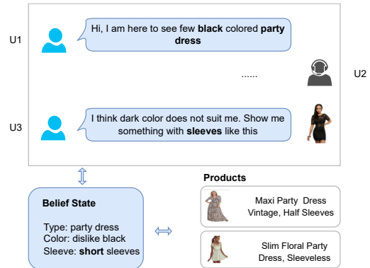
Figure 1: In a multimodal CRS, a user expresses her/his requirements with preferred example image. The dialog state (belief state) encapsulates user interest across turns and modalities.
