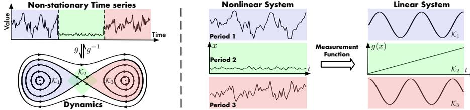
Figure 1: The measurement function  $g$  maps between non-stationary time series and the nonlinear dynamical system so that the timeline will correspond to a system trajectory. Therefore, time series variations in different periods are reflected as sub-regions of nonlinear dynamics, which can be portrayed and advanced forward in time by linear Koopman operators  $\{\mathcal{K}_1, \mathcal{K}_2, \mathcal{K}_3\}$  respectively.
