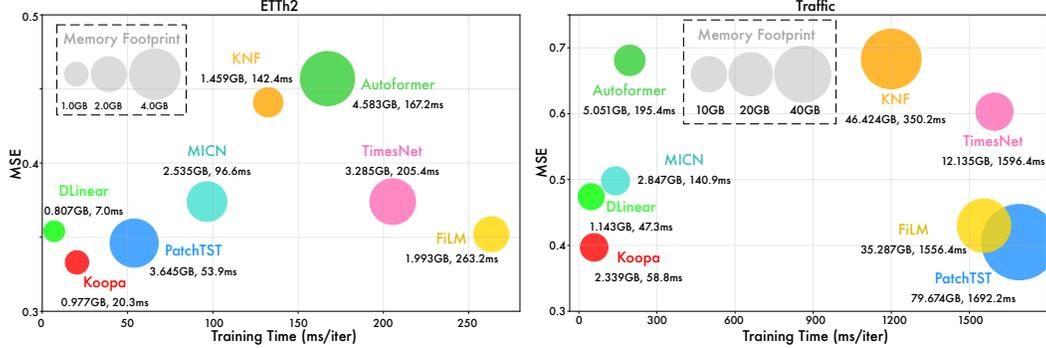
Figure 4: Model efficiency comparison. The performance comes from Table 1 with forecast window length  $H = 144$ . Training time and memory footprint are recorded with the same batch size and official code configuration. Full results of all six datasets are provided in Appendix D.3.
