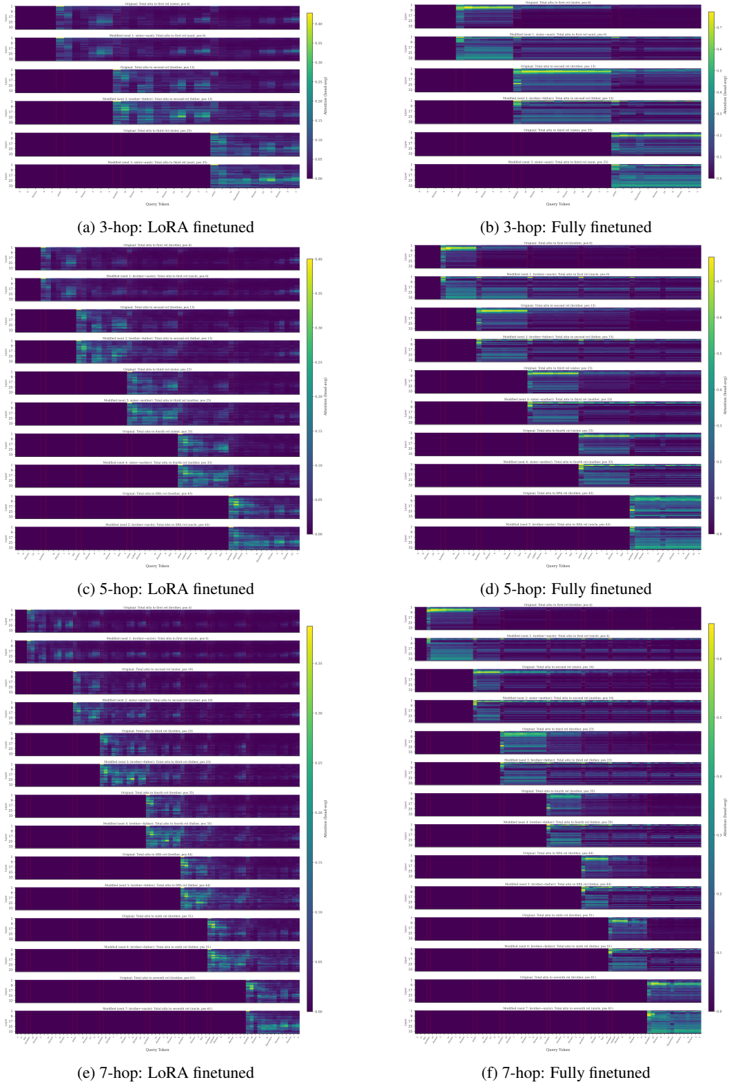
Figure B9: Attention to key token t^r by layer and query token for the causal patching examples of GPT2-large. Attention patterns differ between sibling and mother/father/uncle/aunt relations (first and second row of each location), more markedly so for the fully finetuned models.
