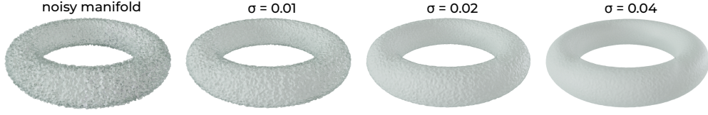
Figure 9: Visualization of the denoising effect for different choices of \sigma . Left: Noisy surface of unit diameter taken as \mathcal{Z} . Second left to right: Image \Pi_\sigma(\mathcal{Z}) under learned projections for different values of \sigma \in \{0.01, 0.02, 0.04\} . A larger choice of \sigma leads to a projection onto a smoother surface.
