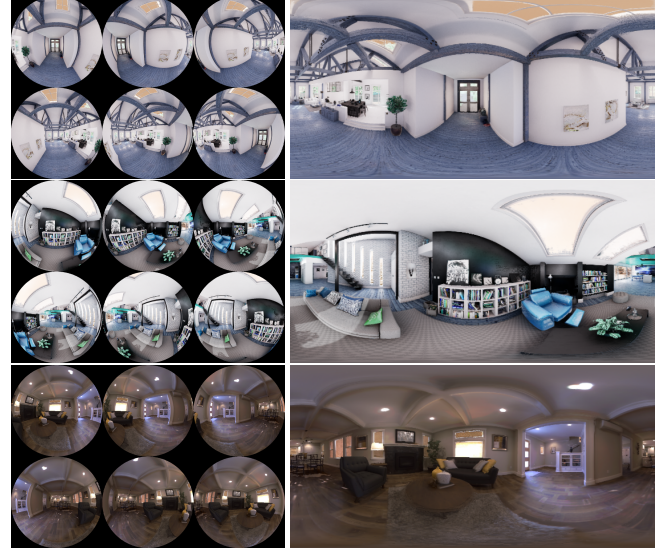
Fig. 5: Illustration of system input and output. Left column: Input fisheye images. Right column: Render result from MSI predicted by our system.
