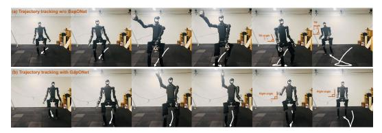
Figure 4: **Locomotion trajectory tracking.** (a) shows trajectory tracking using PD control, where the path (white line) deviates significantly, and the robot's torso tilts drastically, indicating instability. (b) shows the full-body motion after upper-body correction with **GapONet**. Although there is still some rightward deviation, the trajectory is much more stable, and the robot's torso remains upright.
