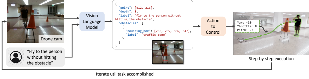
Figure 2: Pipeline overview. A camera frame and user instructions enter a frozen vision-language model, which returns a structured JSON with a 2D waypoint and any obstacle boxes. An Action-to-Control layer converts this output into low-level velocity commands (yaw, throttle, pitch) that steer the UAV. The loop repeats until the task is completed.
