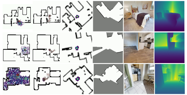
Fig. 2: Tracking (top), semi-global (mid) and global (bottom) localization tasks. From left: a) initial particle distribution b) global map and trajectory with estimated (green) and ground truth (red) poses at each step. Circles denote the final poses. c) local belief map observed by the RL agent d) occupancy grid e) RGB and f) depth.
