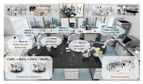
Figure 1: The **LabUtopia** simulation environment and benchmark for developing scientific embodied agents in automated laboratories. LabUtopia supports **chemical reaction** modeling and provides **diverse laboratory assets**, forming a high-fidelity testbed for **tasks of varying difficulty**—from atomic actions to long-horizon action sequences involving both manipulation and navigation.
