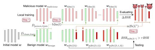
Figure 2: Identifying BC layers with Layer Substitution Analysis. b2m(l) indicates inserting the l,-th layer in the benign model to the malicious model,  $m2b(L^*)$  indicates inserting the malicious model's layers within the subset  $L^*$  to the benign model, and BSR indicates Backdoor Success Rate.
