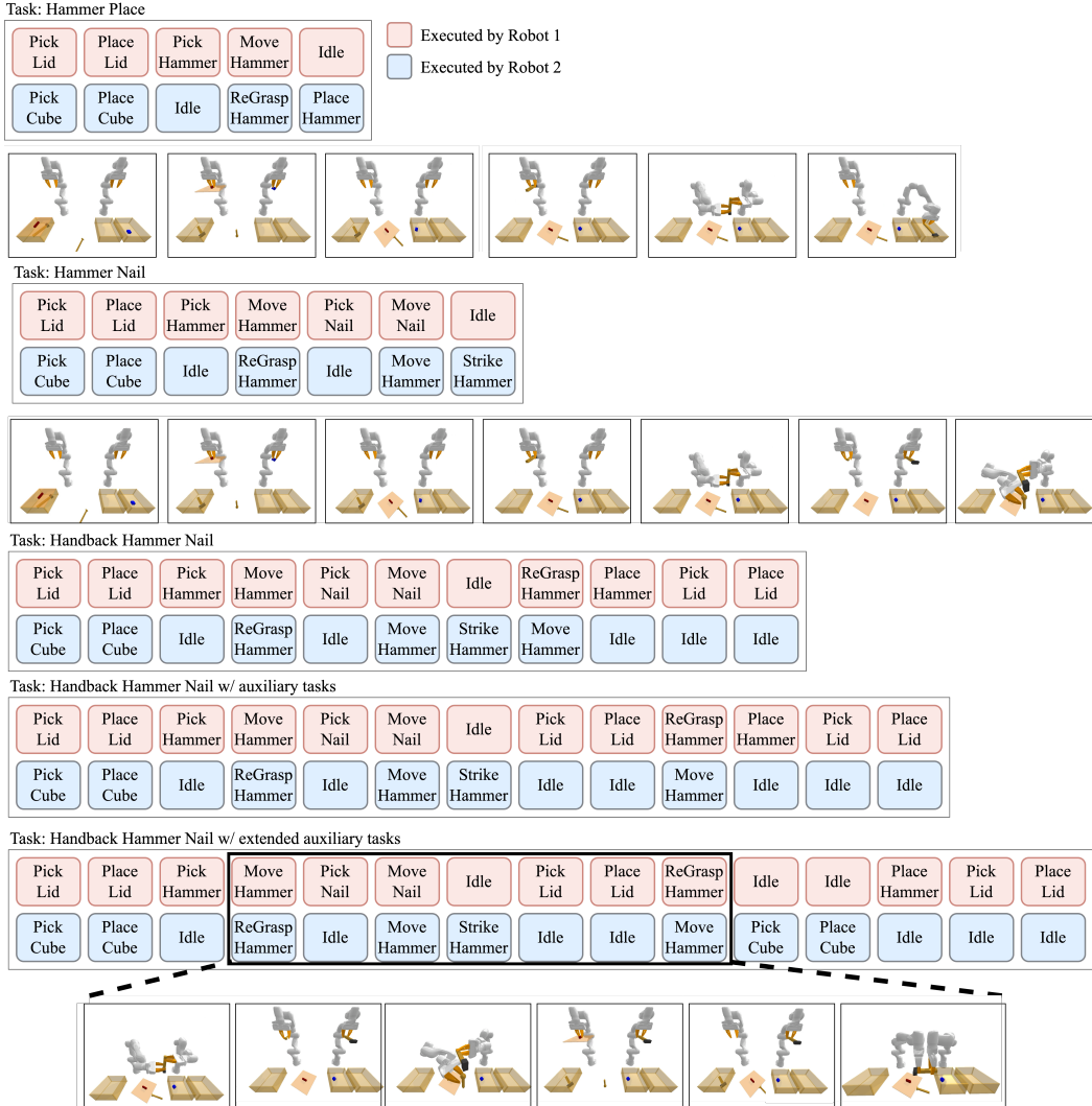
Figure S16: Extension of Hammer Nail task. We have added three new extensions to the Hammer Nail task. All of the new tasks focus on handling a second handover. The nature of the first handover adds further constraints into possible ways to perform the second handover. Further, we add task-irrelevant skills in between the plan skeleton to evaluate the robustness of GFC and the spatial-temporal factor graph plan representation.
