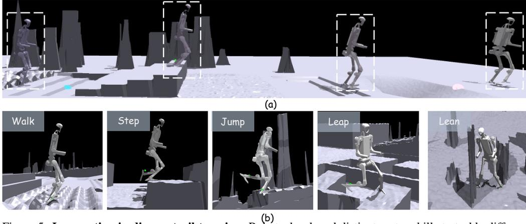
Figure 5: **Locomotion in diverse trail terrains.** Robots developed distinct motor skills to tackle different terrains, e.g., walking on rough surfaces/leaping across ditches/leaning away high obstacles.
