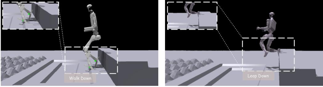
Figure 7: **Motor behavior differences between robots.** Robots with different structures developed unique skills – H1, which is higher and heavier, chooses to “walk down” step, while G1, which is shorter and more lightweight, chooses to “leap down” the step.
