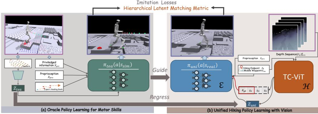
Figure 2: **LEGO-H framework overview.** LEGO-H equips humanoid robots with adaptive hiking skills by integrating navigation  $\mathcal{H}$  and locomotion  $\mathcal{E}$  in a unified, end-to-end learning framework (b). To foster the versatility of motor skills, we train the unified policy via privileged learning from the oracle policy (a).
