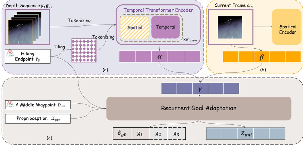
Figure 3: **TC-ViT Architecture.** Three key components: **a)** a goal-orientated temporal transformer encoder for robots cognizing surroundings with the final goal; **b)** a parallel process on the current depth frame for integrating spatially precise information to reflect the current state **c)** a recurrent goal adaptation mechanism that integrates visual awareness, goal information, and proprioception.
