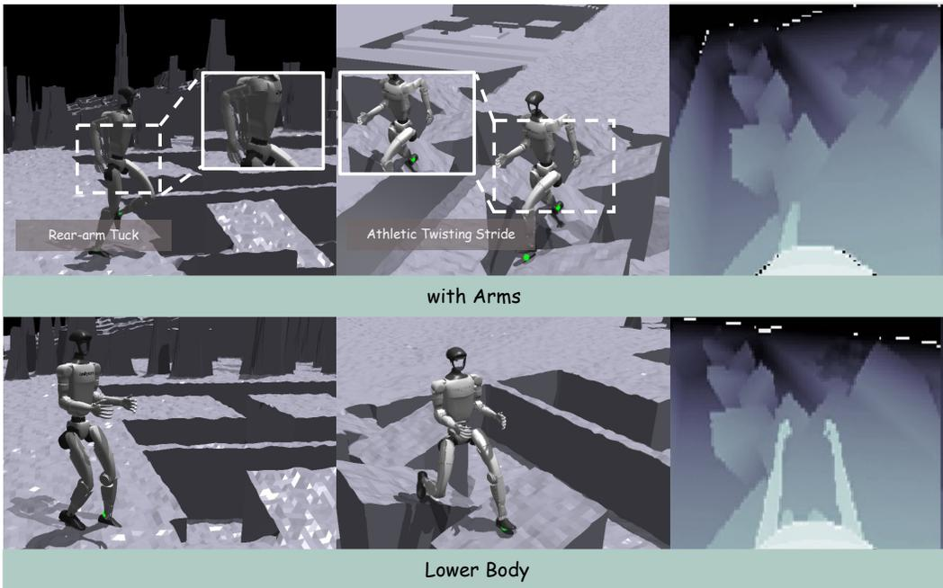
Figure 9: **Preliminary observations for future work on Whole-body Control setting.** G1 exhibits distinct motor behaviors over *with arms* vs *only lower body*. Besides, G1 emerges a rear-arm tuck posture while walking, likely to minimize arm interference with vision (see depth map).
