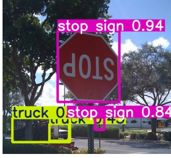
Figure 2: (Second Stage) Final output boxes selected by NMS include the corresponding label and its confidence score.
