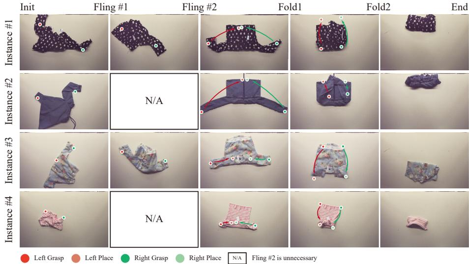
Figure 3: The figure illustrates the shape transformations of different types and sizes of clothes after applying each primitive action of the UniFolding system under various initial states.
