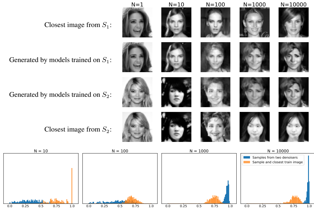
Figure 12: Convergence of model variance. BF-CNN denoisers are trained on non-overlapping subsets S_1 and S_2 of CelebA HQ dataset. The subset size N varies from 1 to 10^4 . See caption of Figure 2.
