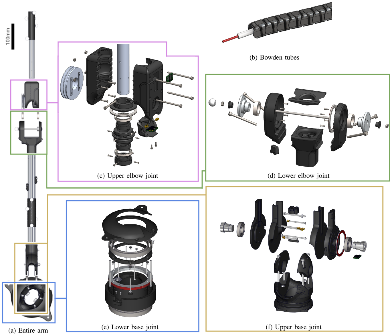
Fig. 2: Design of the tendon-driven robot arm (a). The arm has a rotational and a swivel DoF within the first (e), (f), and second joint (c), (d). It features ball bearings, which are low in friction. Many parts are self-designed and 3D-printed, which are shown colored in black. The four angle encoders are shown with a small green circuit board. The bowden tubes (b) guide the tendons from the muscles to the joints. They feature an inner tube and outer support elements that help maintain constant tendon length.
