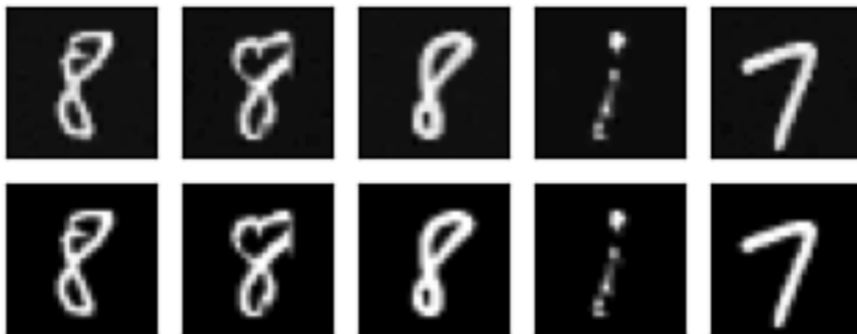
Figure 9: Example of reconstructed MNIST images using the wavelet basis. Top row: reconstructed images. Bottom row: ground truth images. To reconstruct images we use 500 measurements and the number of layers optimized to get the best reconstruction possible.
