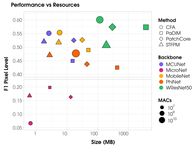
Figure 1. We show on the x-axis the inference time and on the y-axis, the performance. Each color represents a different AD method, while each symbol represents a different tiny backbone. The size represents the total memory required.
