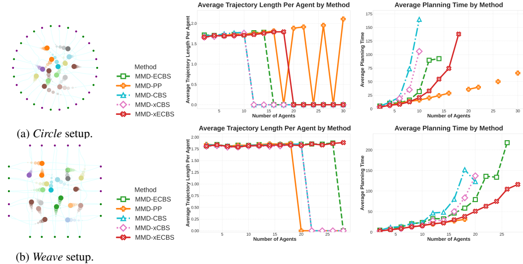
Figure 4: Scalability tests in high-congestion free-space MRMP. Circle (top row) asks robots to swap positions between opposite points on the perimeter. Weave (below), asks robots to exchange positions along uniformly spaced boundary points. Length is zero for failed problems (MMD-PP failures were due to yielding invalid solutions, and other methods failed by exceeding 240 seconds).
