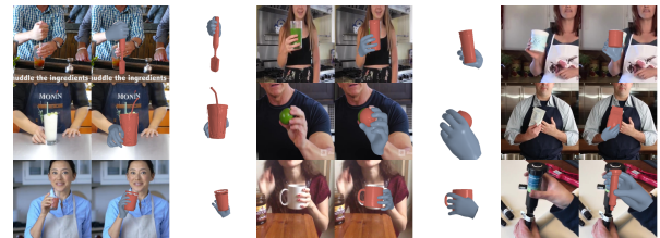
Fig. 4: Our approach applied to in-the-wild images from the 100 Days of Hands dataset [36]. For each image, we estimate 3D hands using HaMeR [17], inference object geometry using MCC-HO and retrieve a 3D model using RAR.
