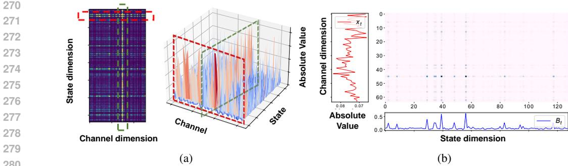
Figure 3: State distribution in Mamba2-370M. **Left:** Outliers exist in both specific state dimensions (red) and channel dimensions (green). **Right:** Further analysis reveals outliers in channel dimension and state dimension can be attributed to variables  $x_t$  and  $B_t$ , respectively.
