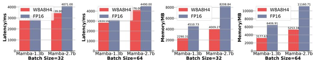
Figure 5: Inference latency and memory usage of the Mamba2 models with different batch sizes on NVIDIA GeForce RTX 3090.
