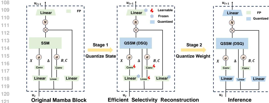
Figure 1: Schematic of the PTQ framework for Mamba. **Left:** The selective parameters  $B$ ,  $\Delta$ , and  $C$ , along with the SSM inputs  $x$ , are generated by the input projections in the Mamba block. **Middle:** After quantizing states using DSQ, ESR updates a small number of selective parameters (approximately 2% of the total) in a block-wise reconstruction manner. **Right:** Finally, we quantize the linear projection into W&A8.
