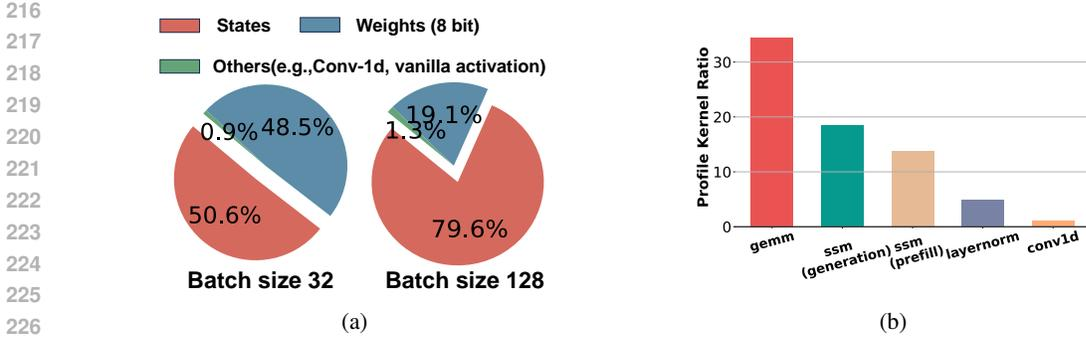
Figure 2: State distribution in Mamba2-370M. **Left:** Memory consumption of weights and state caches in Mamba2-2.7B with different batch sizes. **Right:** The Runtime of the Mamba2-2.7B model using NVIDIA profiling tools, with both prompt and generation lengths set to 100 and a batch size of 32.
