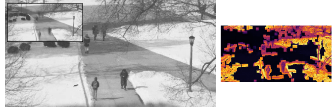
(d) Winter stroll . A slight camera motion results in branches and road outlines also getting sampled at a higher rate in addition to the moving pedestrians. Total detections and measurements are 57% and 53%, respectively, of full data. We used M = 256 and S_{\max} = 16 here.
