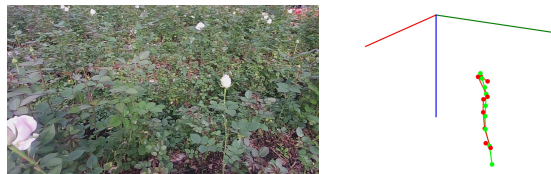
Figure 7: A 3D Rose Localization case. The left shows the original image, and the right shows the spatial reconstruction results from the keypoints. Green result indicates the ground truth, and red result represents the results inferred by ViTPose (Xu et al., 2022) + Depth Anything (Yang et al., 2024).
