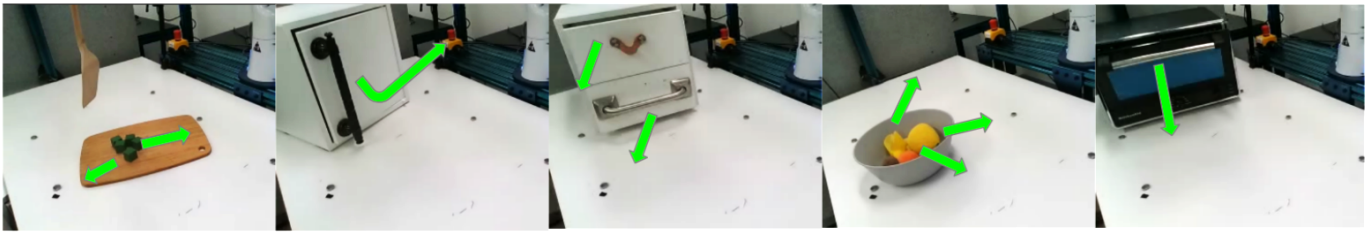
Fig. 7. Figure showing a few configurations of the objects we place in the scene for our experiments, with green arrows denoting plausible motions; from left to right in the top row: a door with a vertical hinge, a bowl of fruits, a chopping board with veggies; in the bottom row: a toaster oven with horizontal hinge, a stack of two drawers, and a vegetable strainer.
