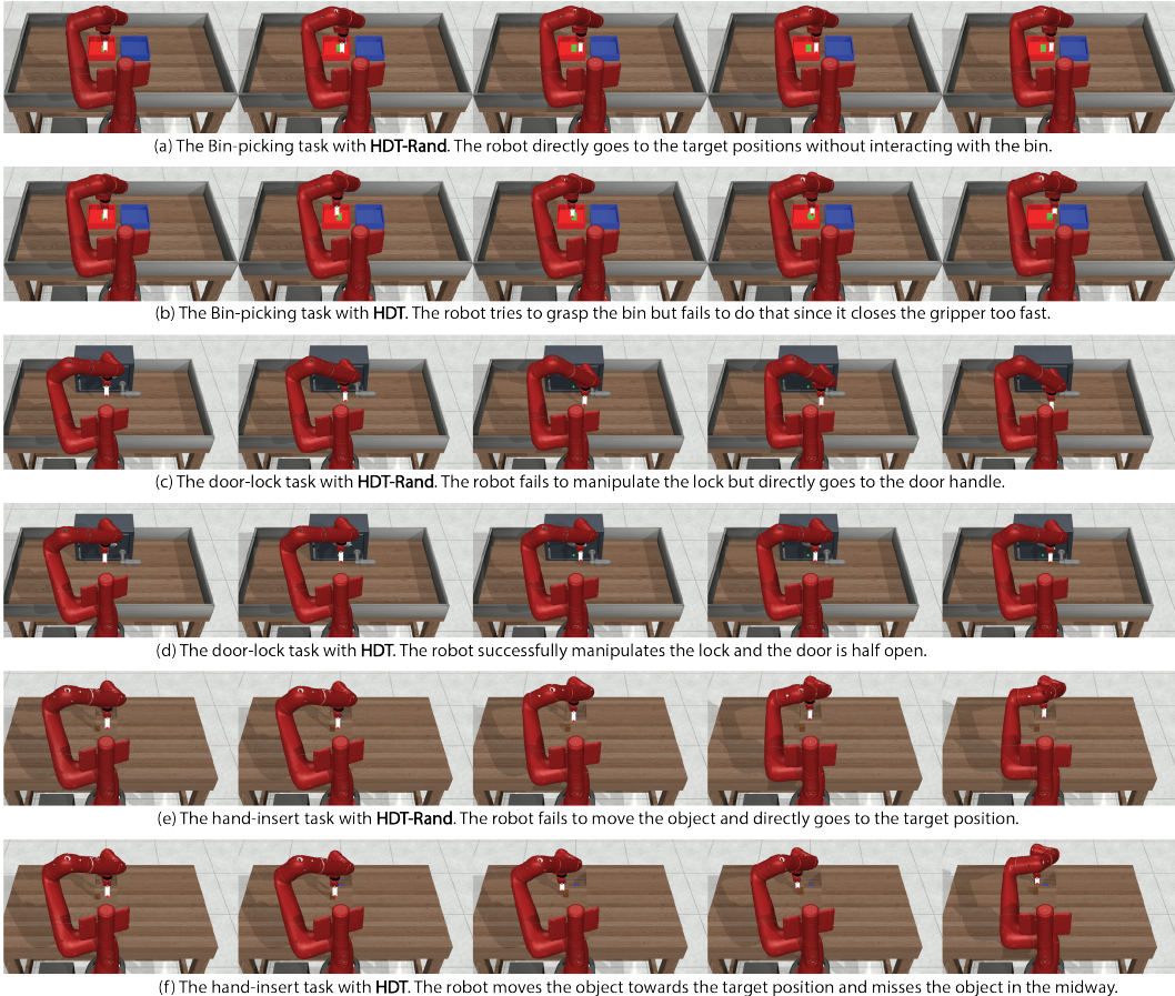
Figure 6: Environment Visualization. We provide key screenshots of three testing environment rollouts to compare the initialization of our proposed HDT and HDT-Rand, which randomly initialize the adapter layers.
