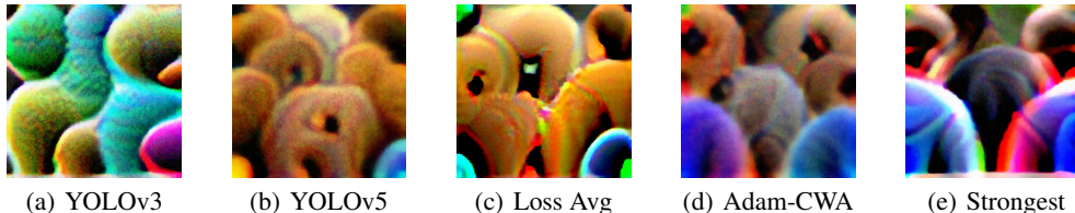
Figure C.1: Visualization of adversarial patches from different methods. The patch simply trained by loss ensemble looks like the fusion of those trained by YOLOv3 and YOLOv5. Adam-CWA captures the common weakness of YOLOv3 and YOLOv5, and therefore generates an completely different patch.
